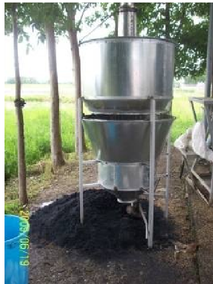
Figure 2: The prototype of the continuous rice hull carbonizer prior to design improvements
