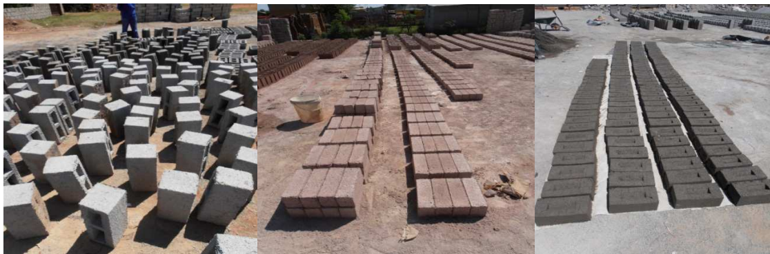
Figure 16: Curing and storage in different sites visited.
