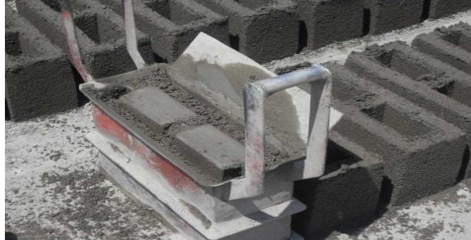
Figure 14: Machine for the production of hollow blocks
