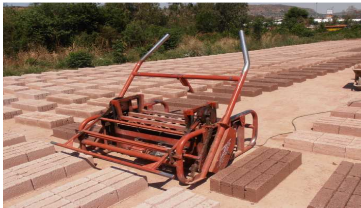
Figure 15: Machine for the production of bricks.
