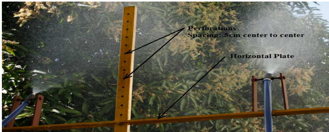
Figure 3: Arrangement of nozzle and horizontal plate resting on a vertical perforated prong.
