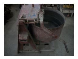
Figure 3: Pan Type Mixture
