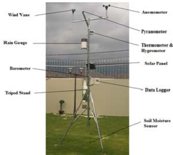
Figure 3: Hobo Weather Station In Yong Peng [4]
