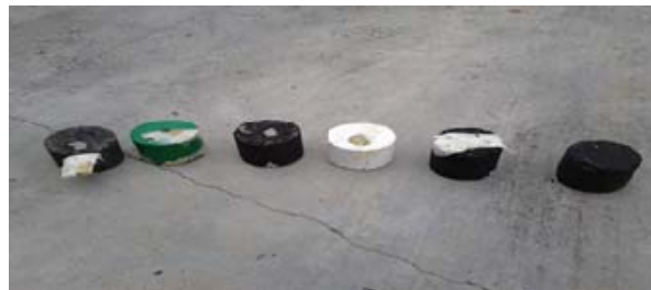
Figure 10: Asphalt Concrete Samples With Different Colours (Albedo)
