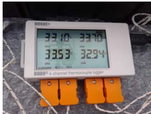
Figure 11: Ux120 Data Logger For Monitoring Thermal Measurements
