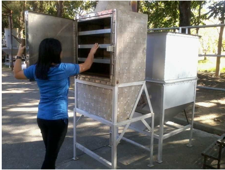
Figure 3. The oven attachment of the CtRH carbonizer.
