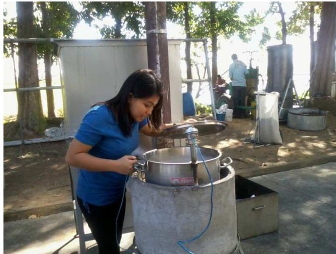
Figure 2. The cooking attachment of the CtRH carbonizer showing the mounted cooking vessel.
