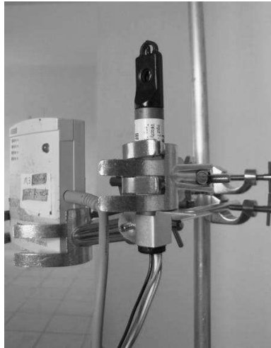
Figure 5 Data logger and sensor for data acquisition
