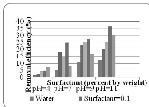
**Fig. 1. Diesel removal efficiency (%) with respect to increasing surfactant amount (Diesel concentration: 10000ppm)**
