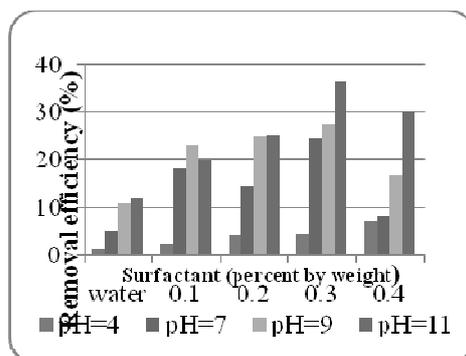
**Fig. 2. Removal efficiencies (%) with respect to increasing pH values (Diesel concentration: 10 000ppm)**
