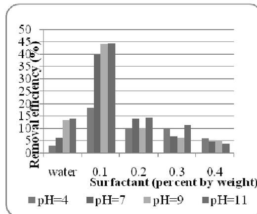
**Fig. 4. Removal efficiencies (%) with respect to increasing pH values (Diesel concentration: 20000ppm)**
