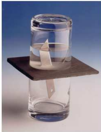
Figure 1: Rapid self-healing character of Liner D - Rawmat HDB (high density bentonite)
