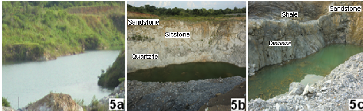
Figure 5: Photograph of abandoned quarry pits in the area, with physically observed rock units corresponding to the electrical resistivity result
