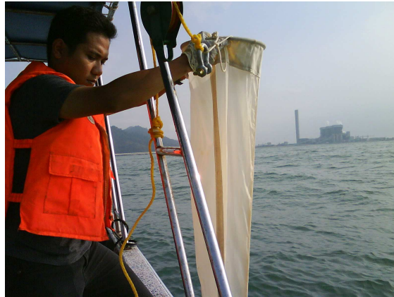
Figure 3. Taking sample using plankton net. In the background shown the coal-fired power station
