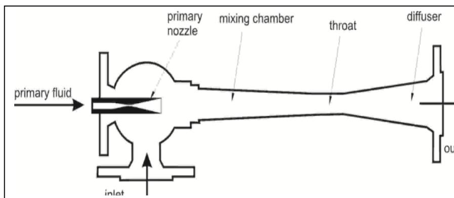
**Figure 5.** Schematic Diagram of a Jet Pump
