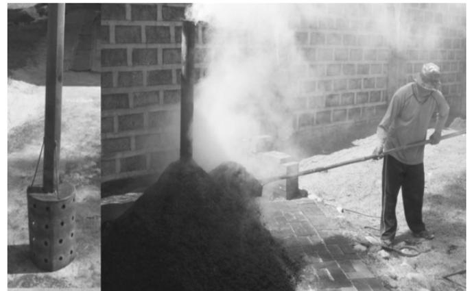
**Figure 4.** The Existing RH Carbonizer Commonly Used by the Farmers.
