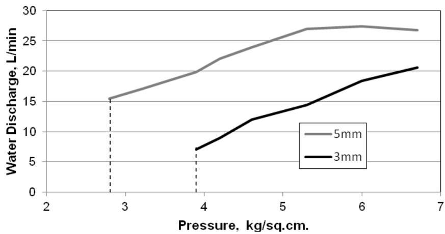
**Figure 9.** Water discharge as affected by nozzle size and steam pressure.
