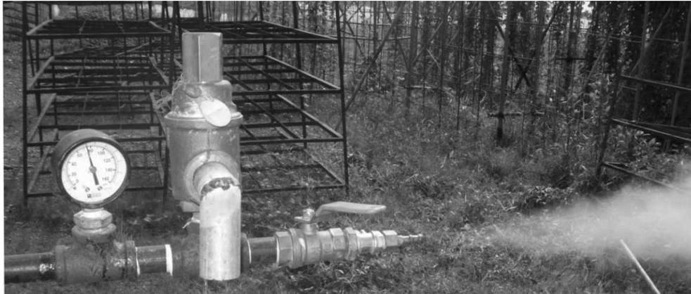
**Figure 8.** The Generated Steam During Laboratory Testing of the Boiler.
