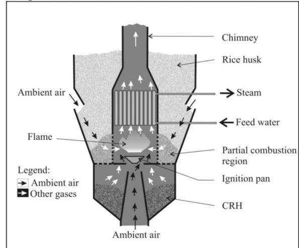
**Figure 3.** The System's Heat Source and Its Heat Recovery Component.
