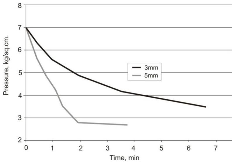
**Figure 7.** Pressure Profile of the System for the Two Nozzle Sizes Used for the Jet Pump.
