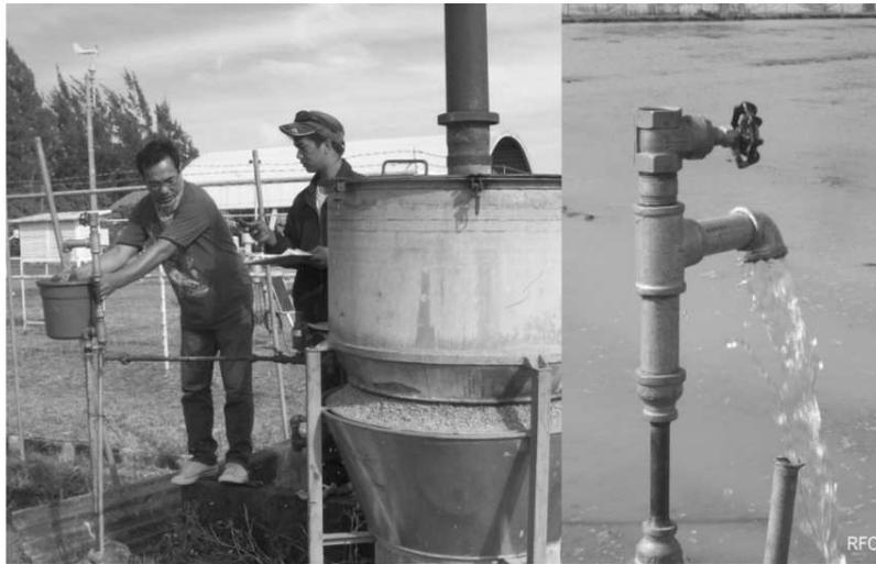
**Figure 6.** The RH Carbonizer-Pump System in Operation Showing a Close up of the Jet Pump (right).
