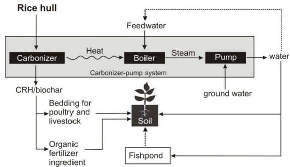
**Figure 1.** The Concept of Utilizing the Carbonization-generated Heat for Pumping Water within the Context of an Integrated Farming System.
