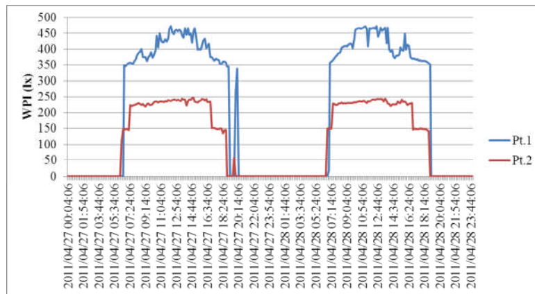
Figure 8: Work plane illuminance(lux) in open-plan office during light on from 27 April to 28 April 2011.
