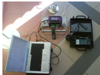
Figure 6: Equipment; Data logger
