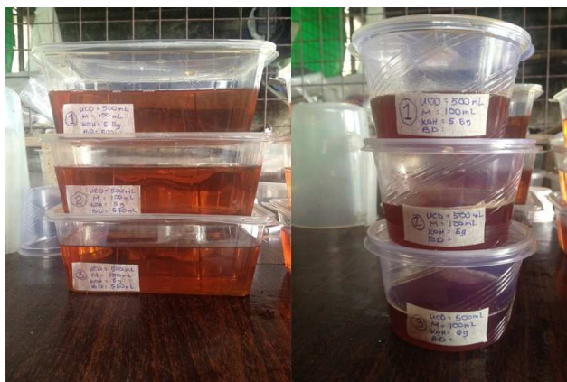
Figure 1. Biodiesel produced from newly purchased (left) and old stacked (right) used cooking oil for the first three treatments.
