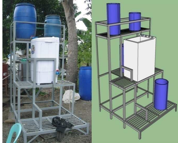
Figure 2. The fabricated and design of the micro-processing plant for biodiesel production
