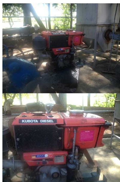
Figure 4. Kubota RK-60 diesel engine used for the test on the different blends of biodiesel
