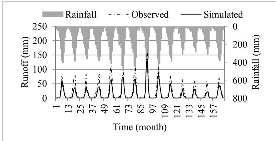
**Figure 4:** Simulated and Observed Average Monthly Runoff Volumes under Land use Scenario E
