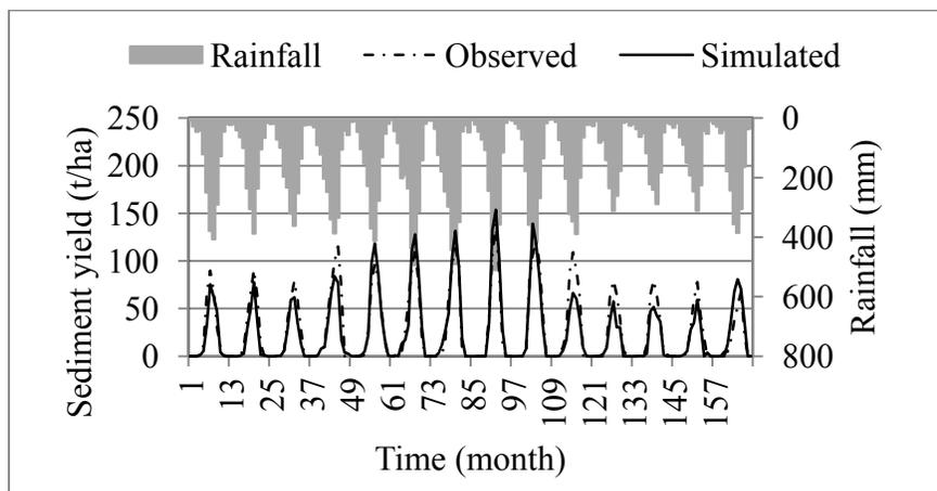
**Figure 6:** Simulated and Observed Average Monthly Sediment Yields under Land use Scenario E
