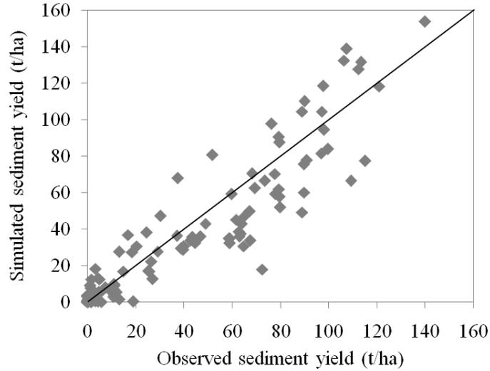
**Figure 7:** Scatter Plot of Simulated vs Observed Average Monthly Sediment Yields under Land use Scenario E
