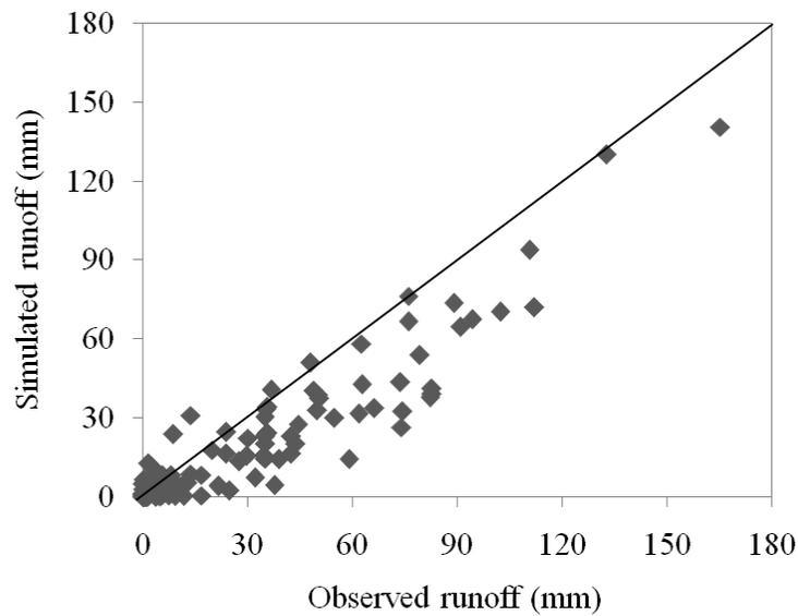
**Figure 5:** Scatter Plot of Simulated vs Observed Average Monthly Runoff Volumes under Land use Scenario E
