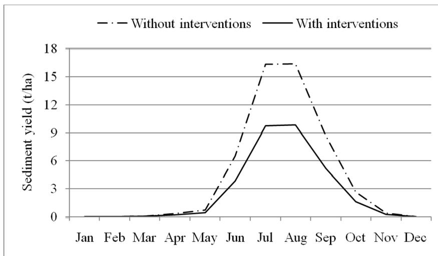
**Figure 10:** Simulated Average Monthly Sediment Yields with and without Soil Conservation Intervention under Land use Scenario B
