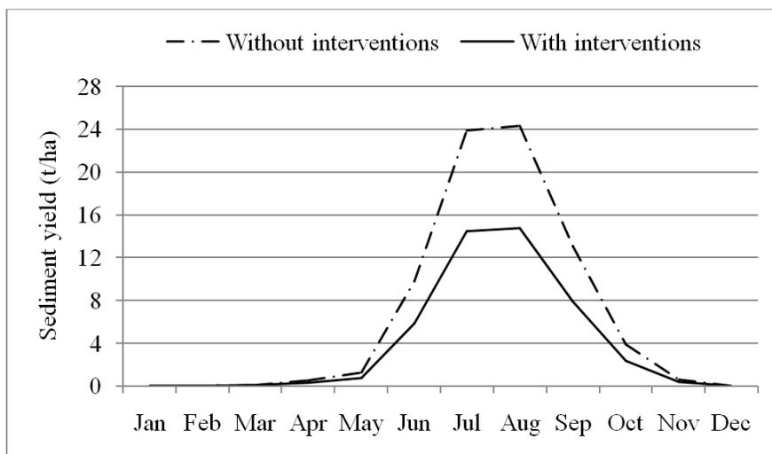
**Figure 11:** Simulated Average Monthly Sediment Yields with and without Soil Conservation Intervention under Land use Scenario E
